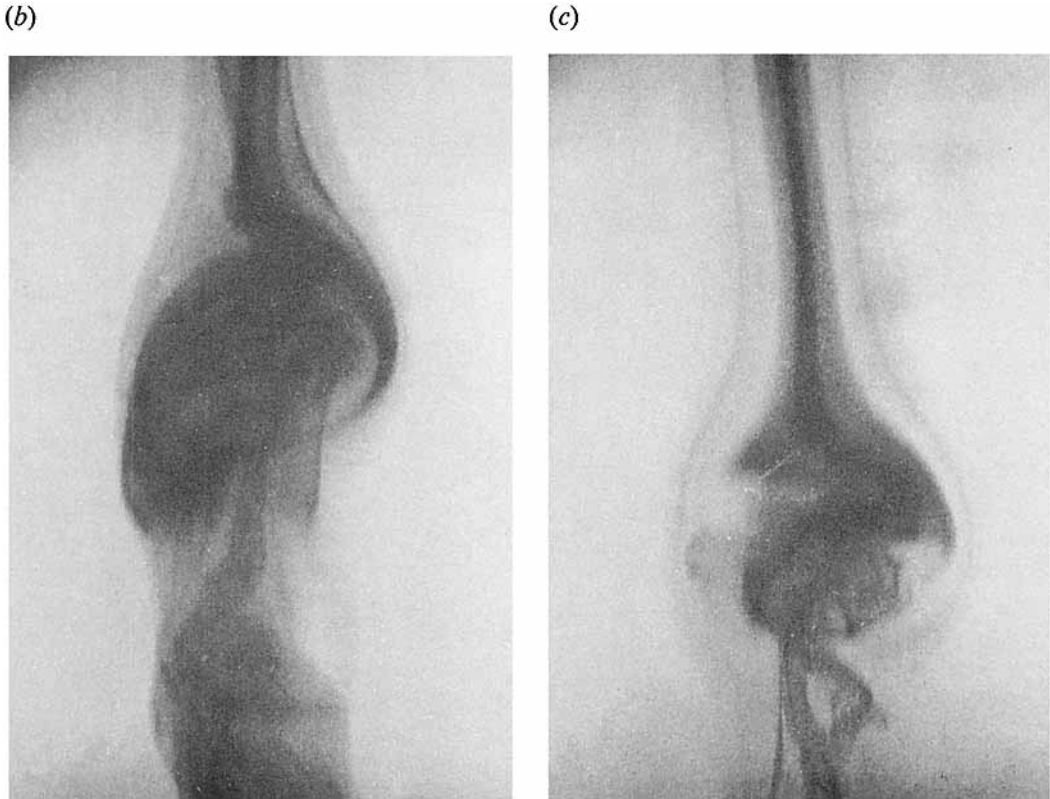
FIGURE 1. (a) Spherical wave propagating along the vortex centreline. Note the laminar wake. \Gamma_\infty = 20 \text{ cm}^2/\text{s} , \xi = 0.73 . (b, c) Vortex breakdown: (b) First stage, \Gamma_\infty = 22 \text{ cm}^2/\text{s} , \xi = 0.77 ; (c) second stage, \Gamma_\infty = 22 \text{ cm}^2/\text{s} , \xi = 0.48 . Shutter speed = 4 \times 10^{-3} \text{ s} , r_0 = 0.635 \text{ cm} .
